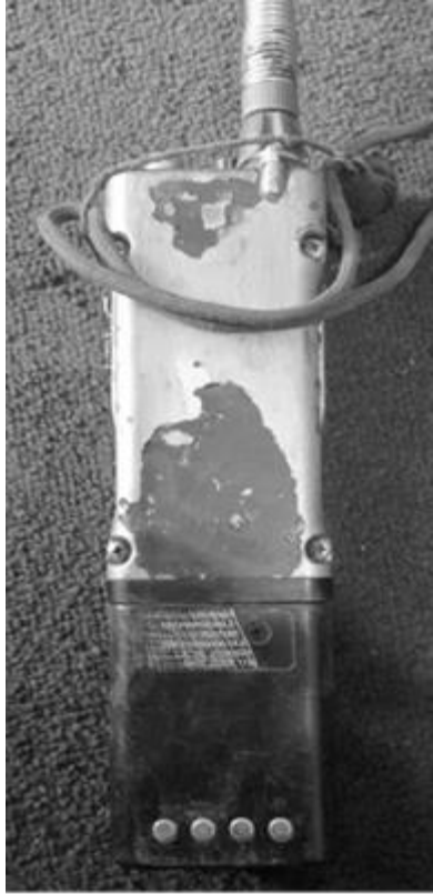
Tadiran RT-7106 (PRC-710) tactical VHF/FM radio transceiver. The attached TEL-718B battery unit is visible at the base. Confidential source
