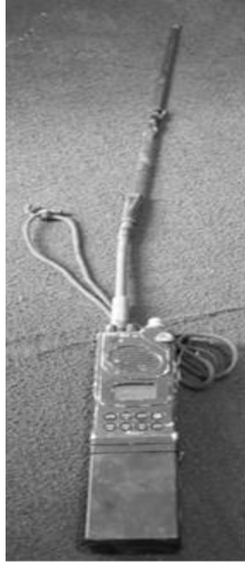
Tadiran RT-7106 (PRC-710) tactical VHF/FM radio transceiver. The attached TEL-718B battery unit is visible at the base. Confidential source
