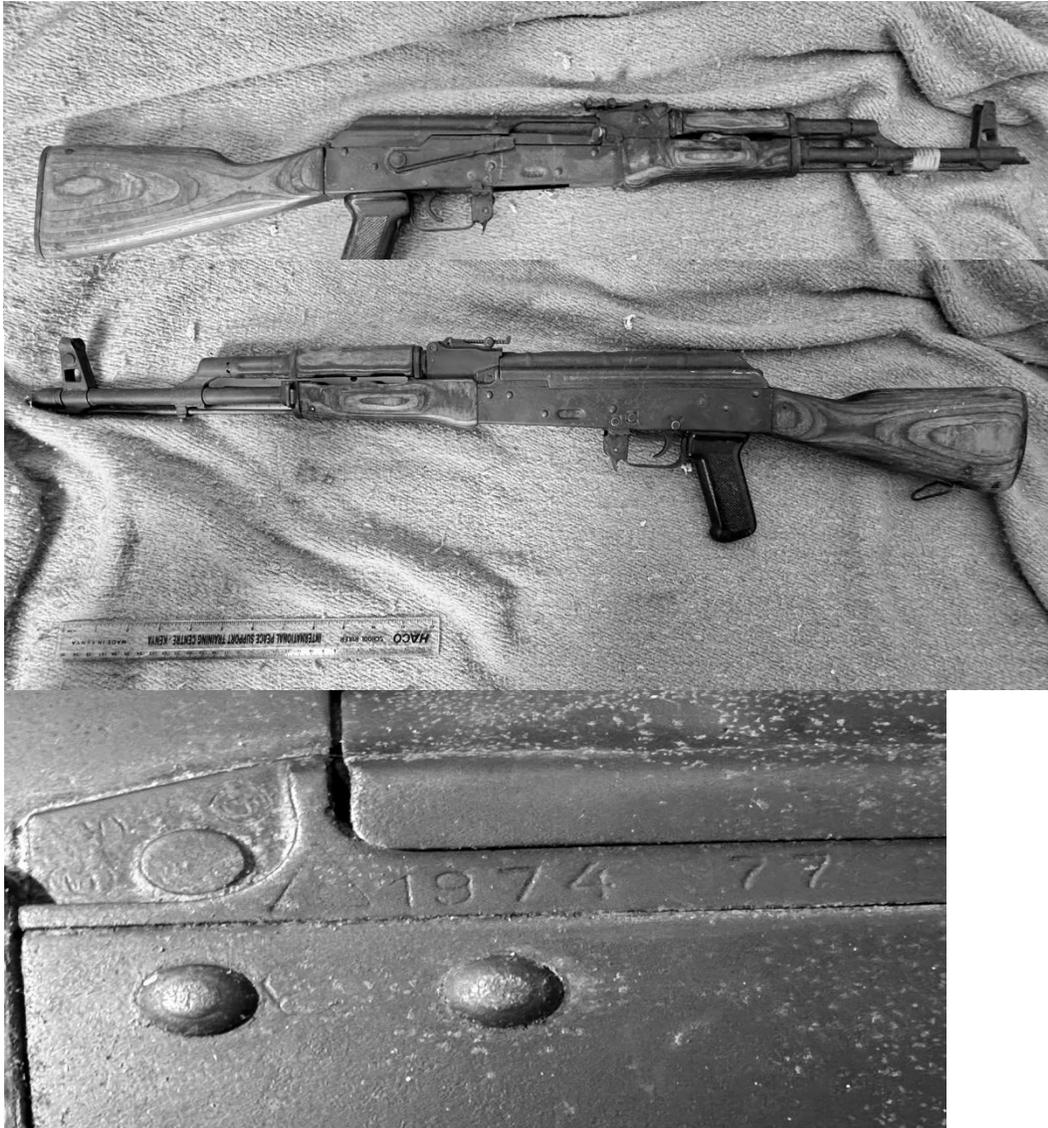
4. One AK-pattern rifle with technical characteristics and factory markings similar to a Type 56 AK pattern rifle chambered for 7.62x39mm ammunition with markings 56 型 (Type) and serial number 40465.
