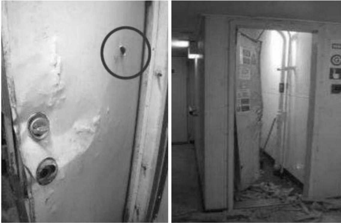
Image 2: The pirates were unable to breach the citadel, but damaged the opening mechanism
