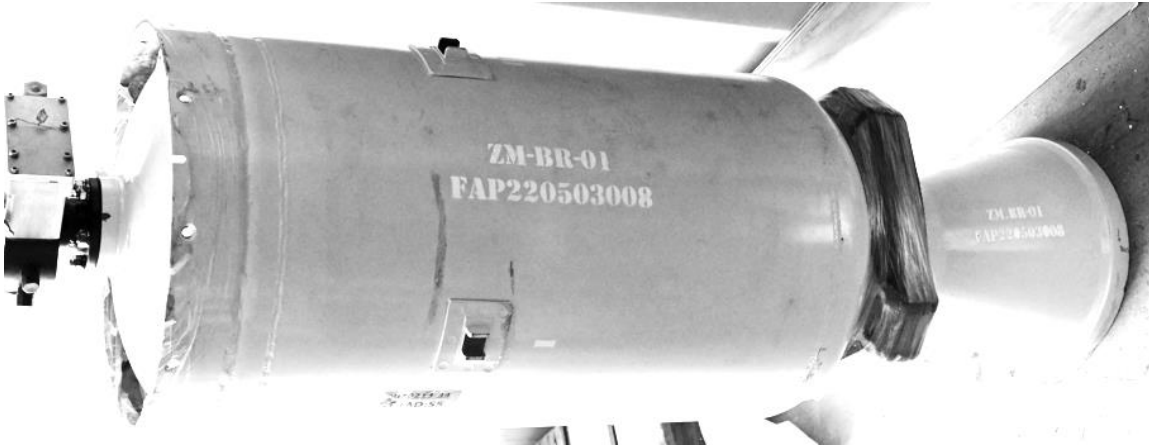
Figure 107.9 Booster, Ghadir ASCM intercepted by the US on 11 January 2024
