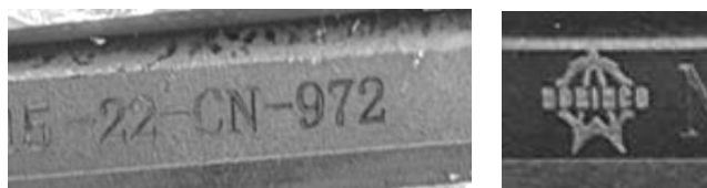
Figure 131.3 (left) 22-CN (2022 as the year of production)
