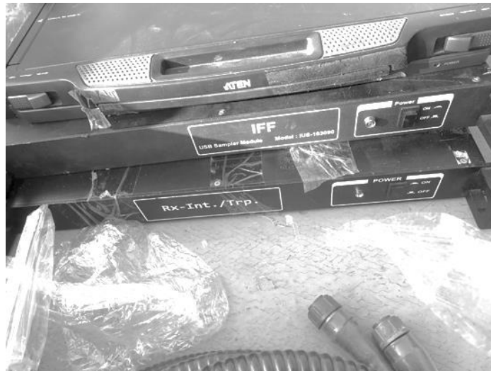
Figures 111.135 (up), and 111.136 (down) USB sampler module intercepted by the US on 28 January 2024
