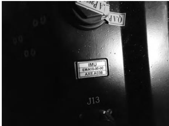
Figure 111.62 SRBM Inertial Measurement Unit (IMU) intercepted by the US on 28 January 2024
