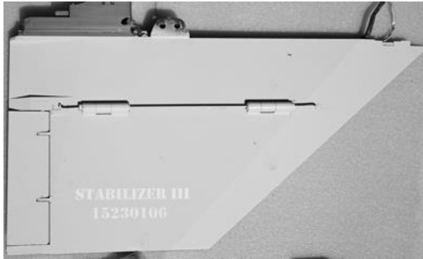
Figure 110.3 Stabilizer, Ghadir ASCM intercepted by the US on 11 January 2024
