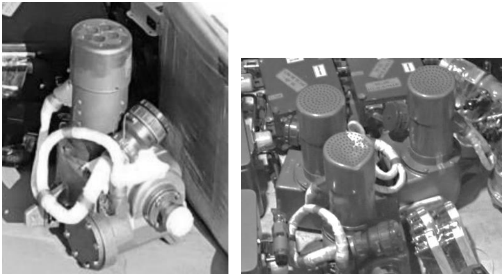
Figures 114.12 (left) and 114.13 (right) SRBM actuators of jet vane control system component intercepted by the US on 28 January 2024
