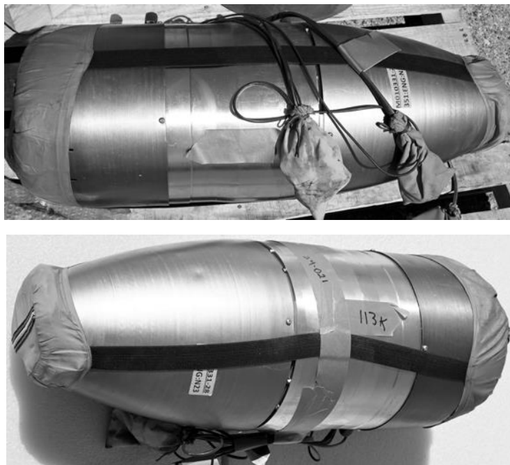
Figures 107.21 (up), and 107.22 (down) Toloue 10 jet engine of « 351 » LACM intercepted by the US on 11 January 2024
