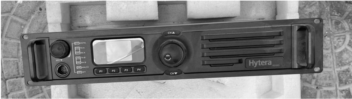
Figure 121.7 VHF station Hytera RD985
