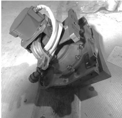
Figures 111.56 (up), 111.57 (middle), and 111.58 (down) SRBM jet vane control system intercepted by the US on 28 January 2024
