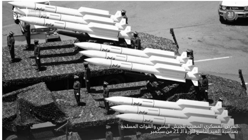
Figure 70.1 Barq-2 SAM operated by the Houthis
