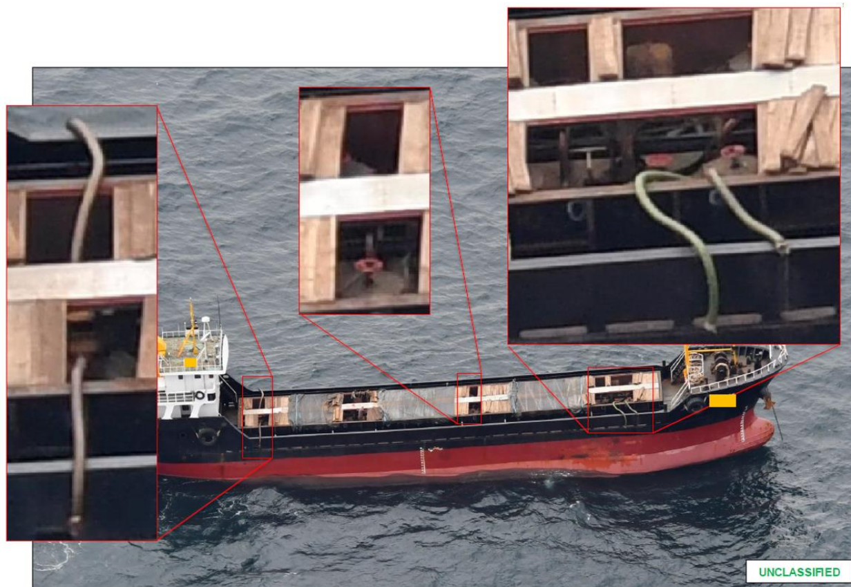
Figure 2: Another example of a re-configured cargo ship with closeups showing likely concealed fuel tanks, East China Sea, October 2020*
