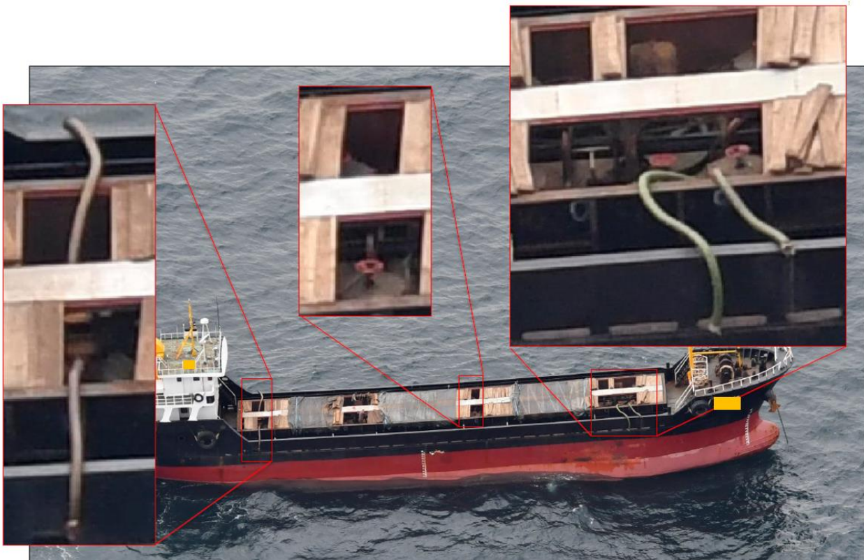
Figure 30: Vessel with closeups showing likely concealed fuel tanks, East China Sea, October 2020*
