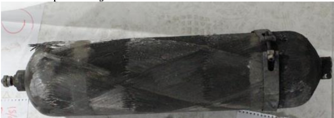
Figure 5.9 Carbon-fibre pressurised gas bottle
