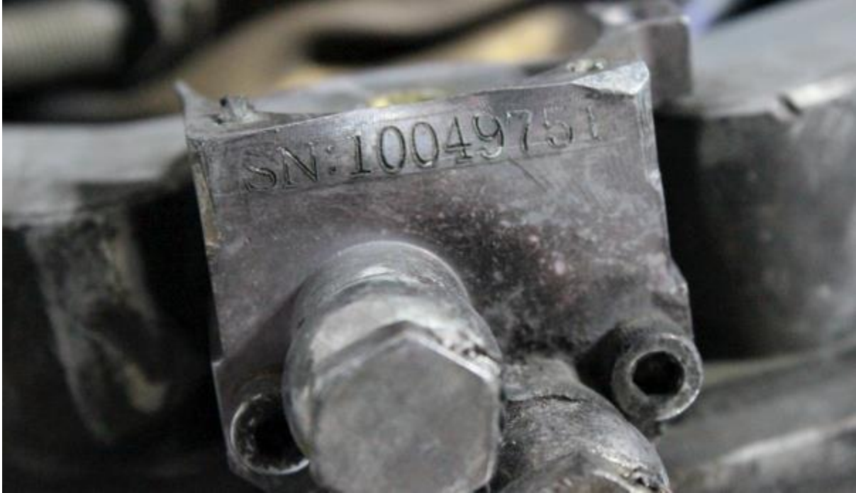
Figure 5.16 Serial number on the debris of the turbojet engine
