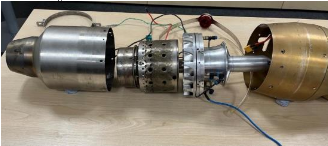
Figure 18.10 Gas-turbine engine of the “358” surface-to-air missile
