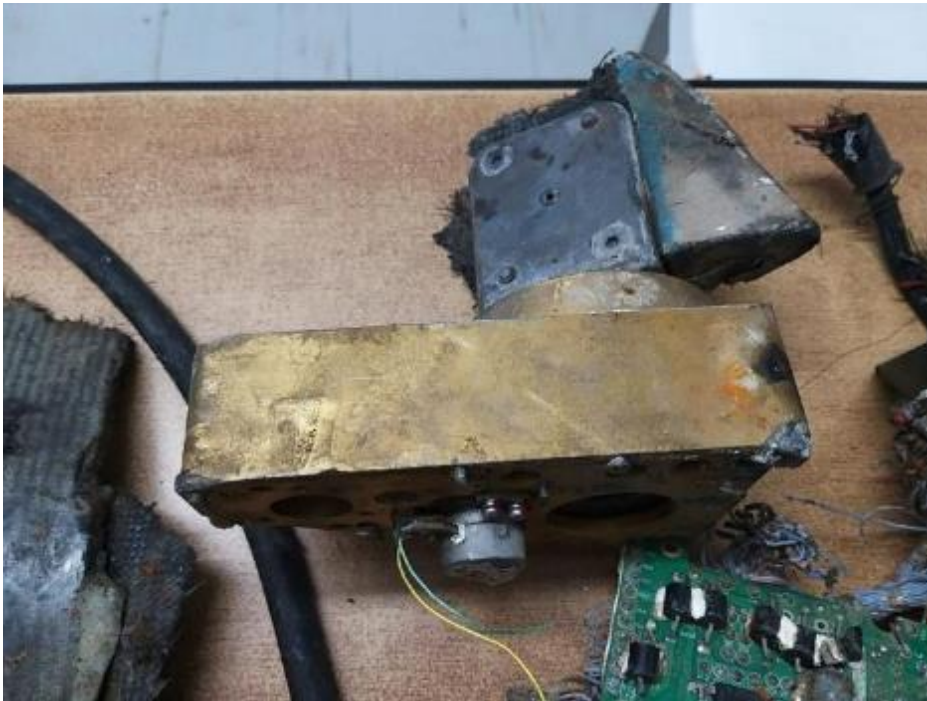
Figure 9.7 Debris of a servo actuator recovered from the seabed after the attack
