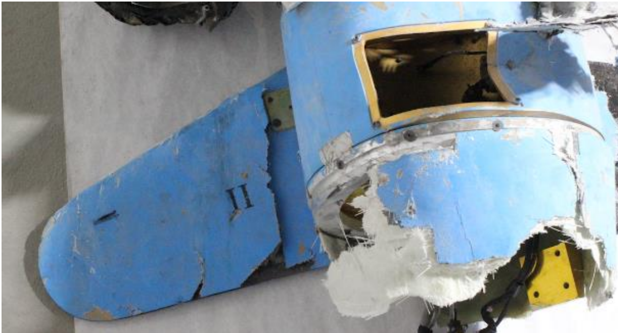
Figure 5.15 Marking on the debris of the control surface of one of the cruise missiles
