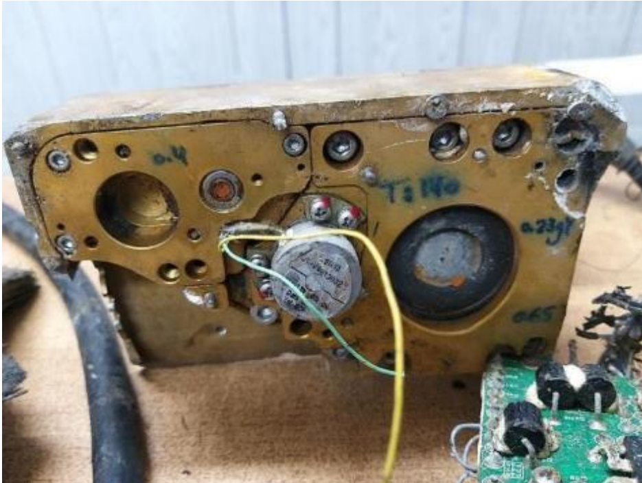
Figure 9.8 Debris of a servo actuator recovered from the seabed after the attack
