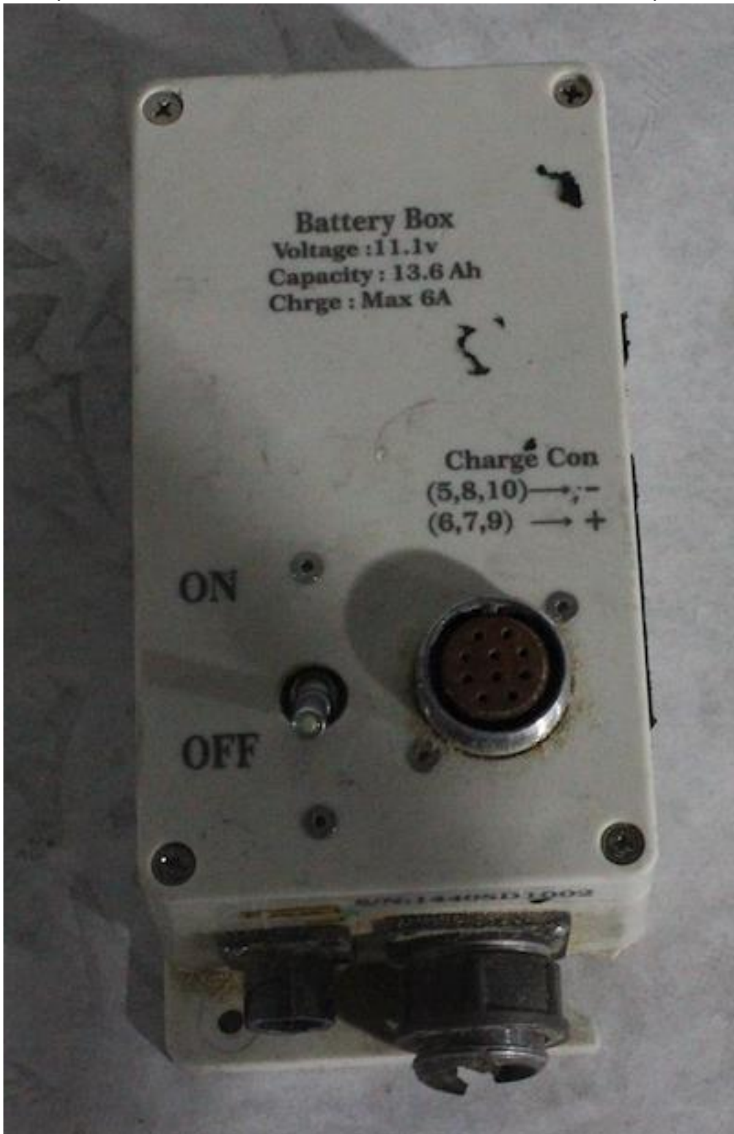
Battery box from one of the “Sammad” UAVs used in the attack on 2 February 2022
