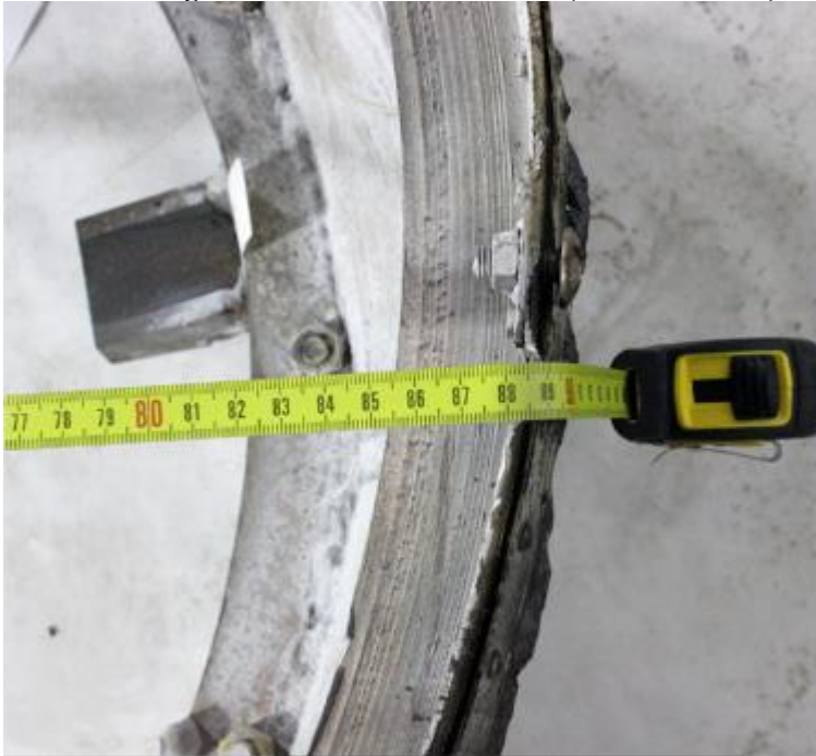
Figure 5.3 Detail showing the diameter of the missile (88 centimetres)
