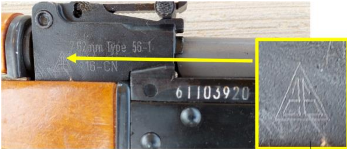
Figure 11.10 Detail of marking on Type 56-1 assault rifle inspected by PoE Somalia
