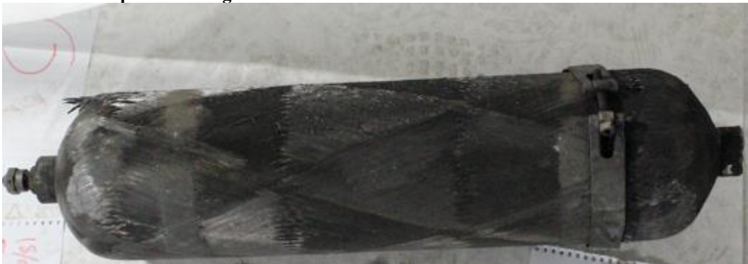
Figure 5.9 Carbon-fibre pressurised gas bottle
