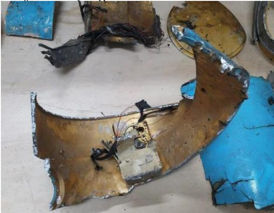
Figure 9.6 Fuselage debris of a Quds-type cruise missile recovered from the seabed after the attack
