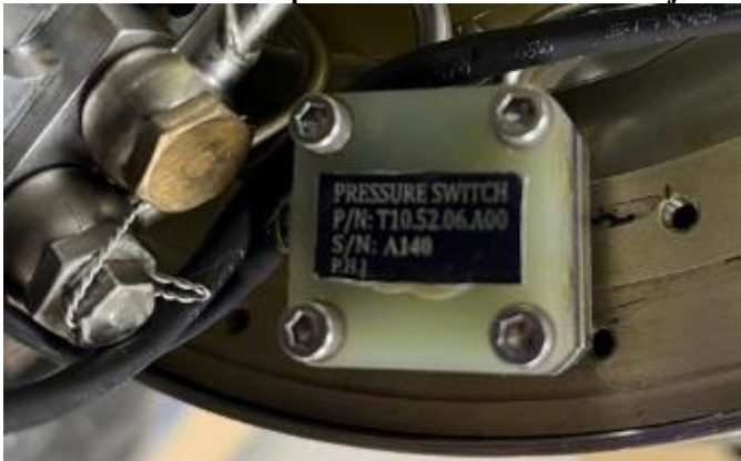
Figure 18.9 Serial number of the pressure switch of the turbojet engine
