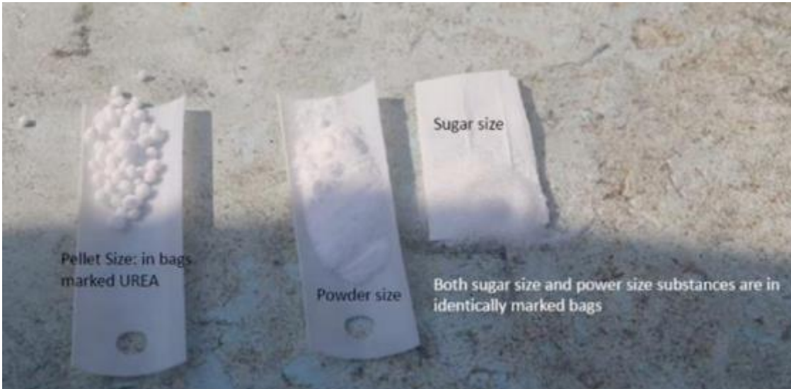
Figure 16.2 Urea fertilizer in pellet form (left), ammonium perchlorate in powder/sugar form (right)
