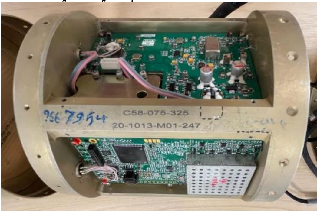
Figure 18.15 Detail of marking on the flight computer
