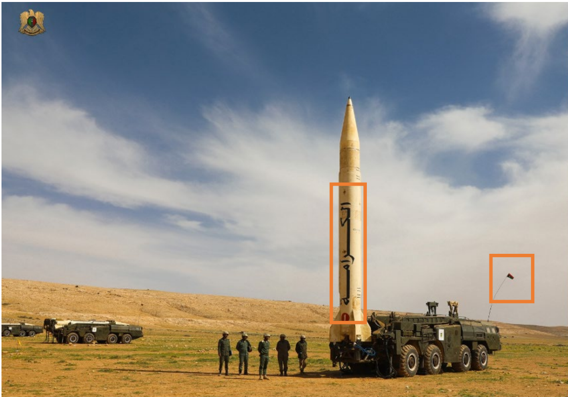
Figure 103.7 TBM on TEL in launch position
