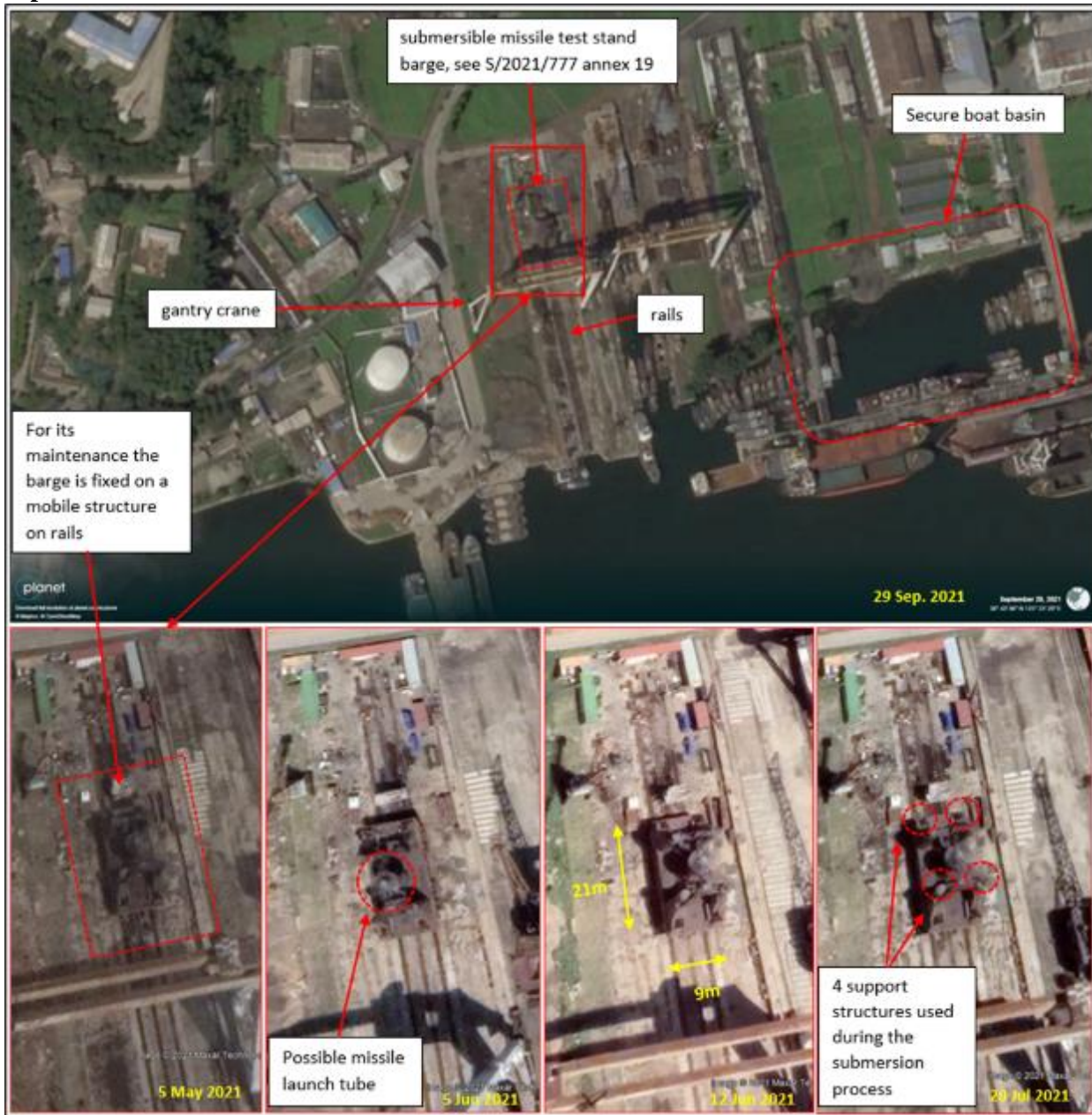
Figure 26-1: Submersible missile test stand barge in Nampo was still under repair or improvement in September 2021
