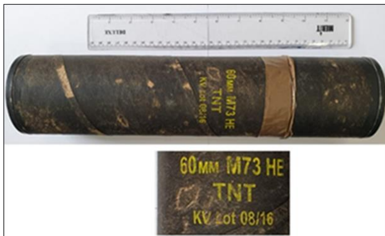
Figure 2: Casing of 60mm mortar round
