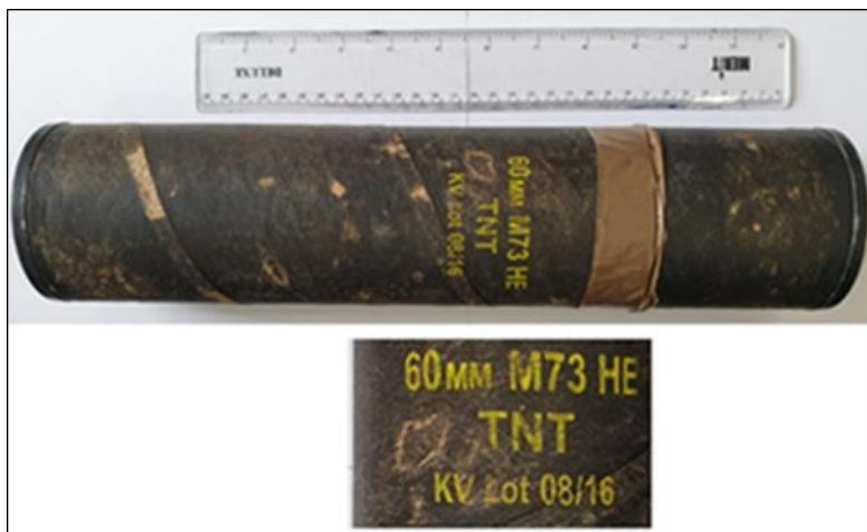
Figure 2: Casing of 60mm mortar round
