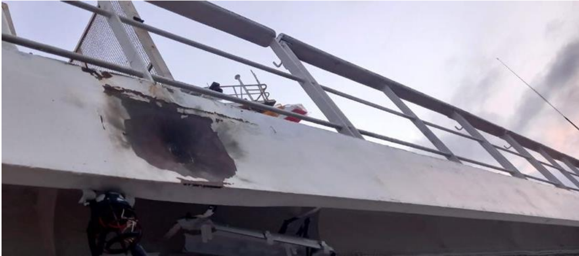
Figure 4: RPG's impact on the vessel.
