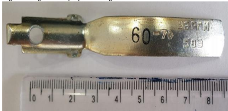
Figure 3: Ignitor cap of a hand grenade.
