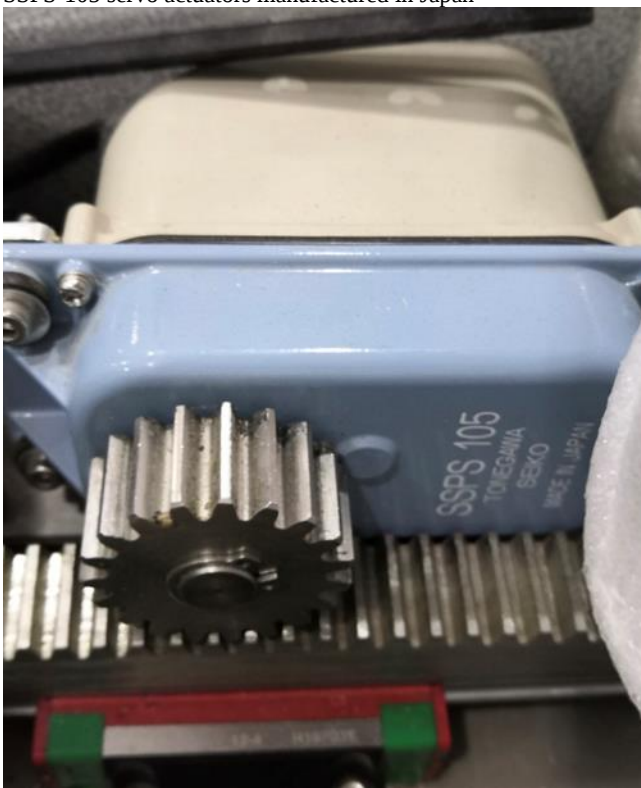
Figure 13.11 SSPS-105 servo actuators manufactured in Japan
