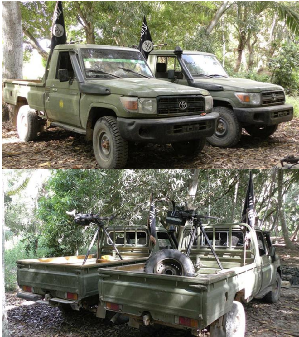
Figures 15 and 16: Toyota pick-up trucks mounted with type 85 anti-aircraft, 12.7-mm heavy machine guns.
