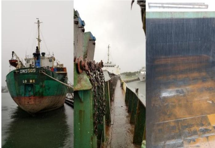
Left: the *DN5505*; middle: traces of coal on the deck; right: the cargo hold.
