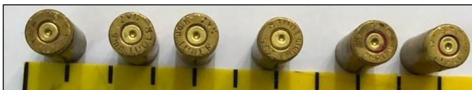
Figure 7: Cases of 9mm bullets with headstamps showing "ZVS 9mm Luger".
