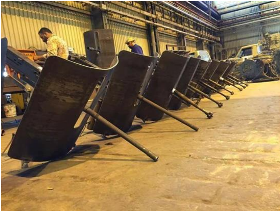
Figure 23 Photograph of LNA workshop in which 12.7-mm and 14.5-mm machine guns with shields are being mounted
