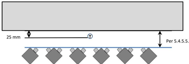
5.5.2. Targeting of the localized and engulfing burner zones on the CHSS
