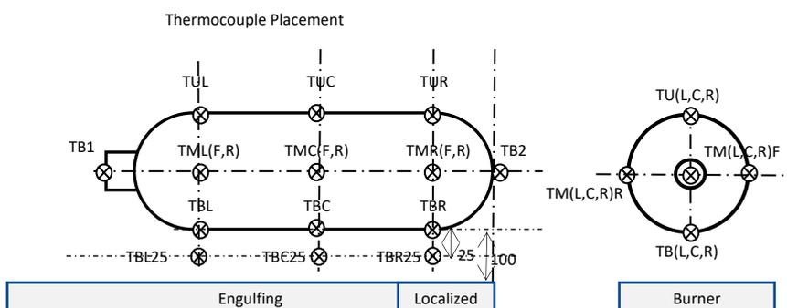
Temperature measurements on the pre-test cylinder shall be performed by  $\phi 3.2$  mm (or less) K-type sheath thermocouples that are located within a 5 mm gap from the pipe surface that are held on the surface by straps or other mechanical attachments. Temperature measurements shown in Figure 5 are defined as follows:
