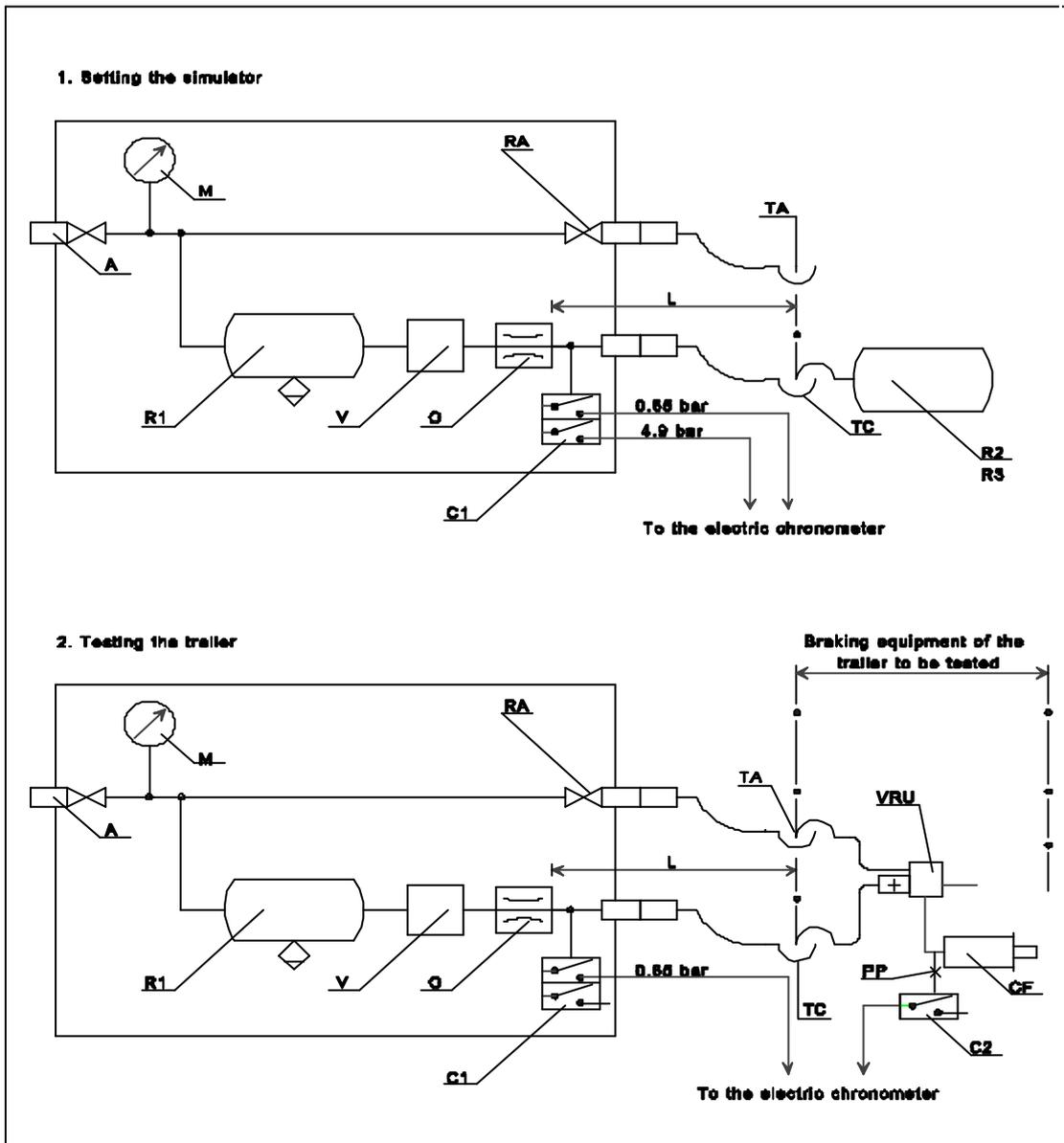
3. Example of a simulator for electric control lines
