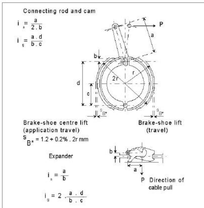
Figure 5: MECHANICAL-TRANSMISSION BRAKING SYSTEM
