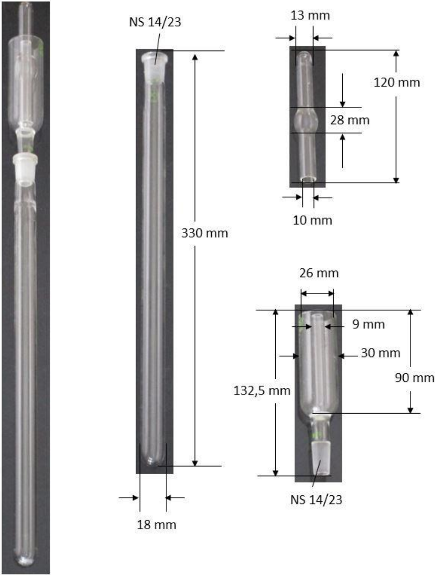
Figure A10.1: Condensing chamber for Bergmann Junk test example 1
