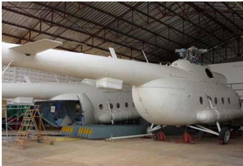
Photo 5: Mi-8T bodies being refurbished in Lomé
