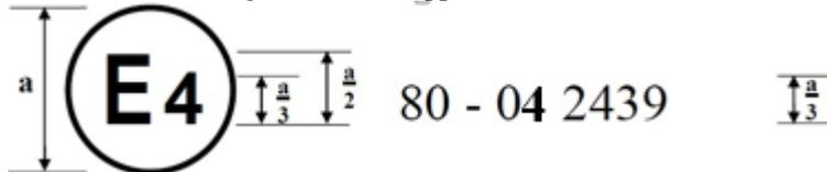
The above approval mark affixed to a seat shows that the seat type concerned has, with regard to the strength of the seats, the test being carried out in accordance with paragraph 2 of Annex 4, been approved in the Netherlands (E4) under number 042439. The approval number indicates that the approval was granted in accordance with the requirements of Regulation No. 80 as amended by the 04 series of amendments.
