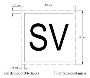
letters "SV" shall be black, a minimum of 120 mm high and have a minimum stroke thickness of 12 mm.
